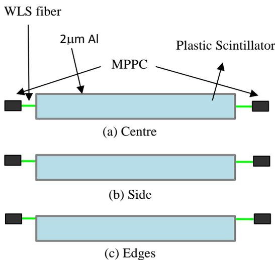
Figure 2: Three Configuration of tested thin
