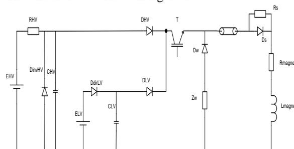
Figure 1: Kickers circuit schematics.
