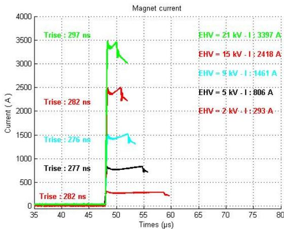
Figure 5: Variable pulse width and amplitude of the extraction kicker.
