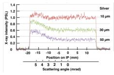
☑ 3: X-ray transmissions through indium and silver foils recorded on the Imaging Plate, IP.
