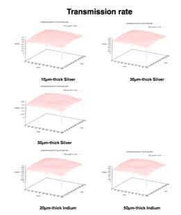
☑ 1: Simulation results of x-ray transmissions through silver foils by using the "CAIN".
