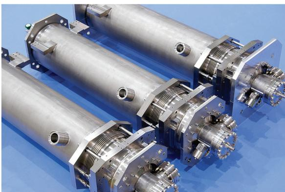
Figure 5 TESLA-shape cavity package hung on the cold mass and the picture of the other three jacketed cavities waiting for installation.
