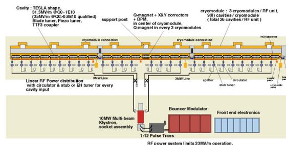
Figure 2 RF unit configuration of ILC main linac.
