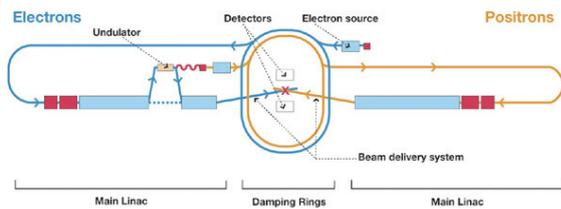
Figure 1 Baseline ILC accelerator configuration
