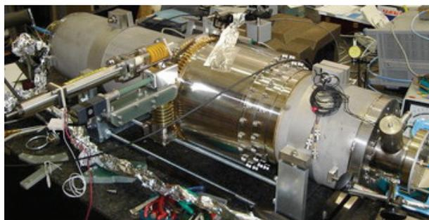
Figure 6 One of the cavity picture of high gradient LL-shape cavity. The test setup of coaxial tuner for LL-shape cavity.
