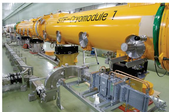
Figure 4 STF Phase 1 cryomodule.
