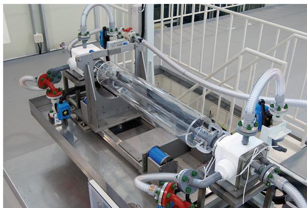
Figure 7 Cavity bed of STF new EP facility. The plastic dummy cavity is mounted for test.
