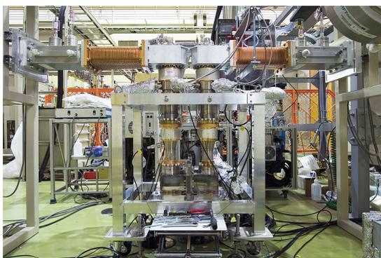
Figure 3 RF power source and input couplers for high power test.
