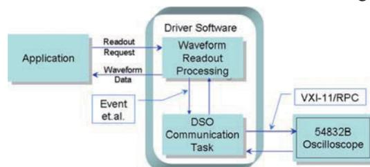
Figure 7: Schematic of Waveform Data Acquisition.
