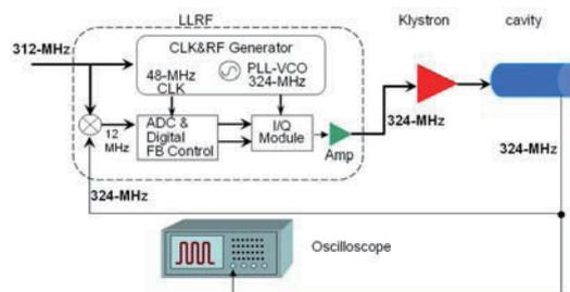
Figure 2: 324-MHz Clock Signal.
