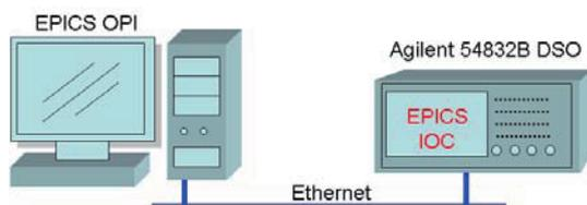
Figure 6: Embedded IOC inside DSO.
