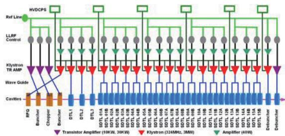
Figure 1: Layout of RF power source of LINAC.
