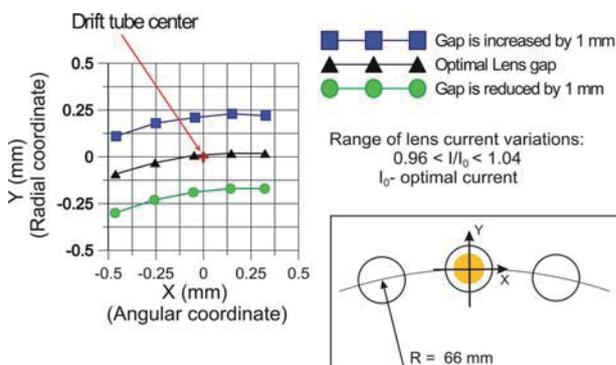
Figure 7. Position of the beamlet center at the compression lens outlet depending on lens current and lens gap size (10 MW L-band klystron case).
