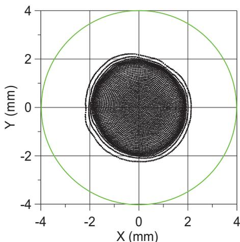
Figure 4. Cross-section of the individual beamlet at the compression lens outlet (40MW X-band klystron case).
