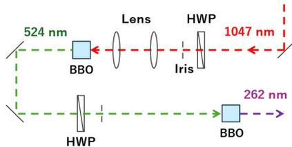
Figure 5: Layout of the fourth harmonic generation.
