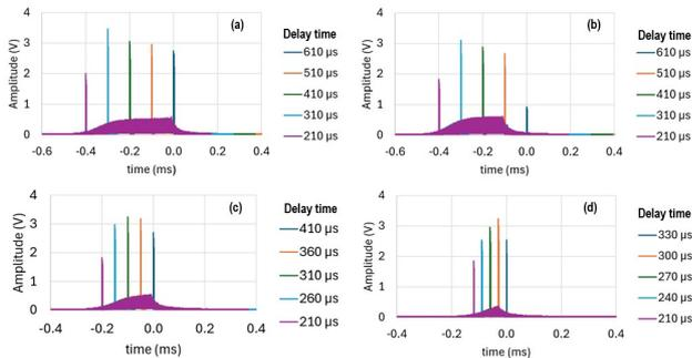
Figure 8: Longitudinal distributions of pump pulse (base) and laser pulse (spikes) from pre-amplifier with different delay times at gate duration of (a)  $600\ \mu\text{s}$ , (b)  $500\ \mu\text{s}$ , (c)  $400\ \mu\text{s}$ , and (d)  $300\ \mu\text{s}$ .
