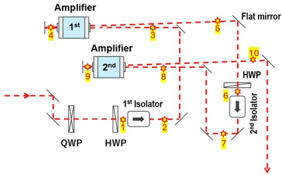
Figure 4: Layout of a Multi-pass amplifier section. Yellow stars with numbers indicate the locations where laser power measurements were performed.
