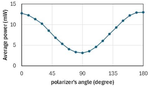
Figure 7: Average power of laser from oscillator after passing through a polarizer with different angles.
