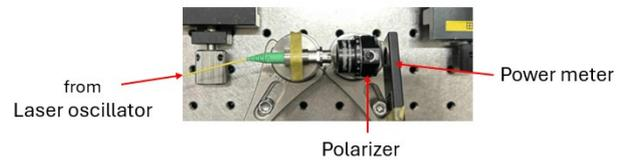
Figure 6: Setup of polarization measurement.
