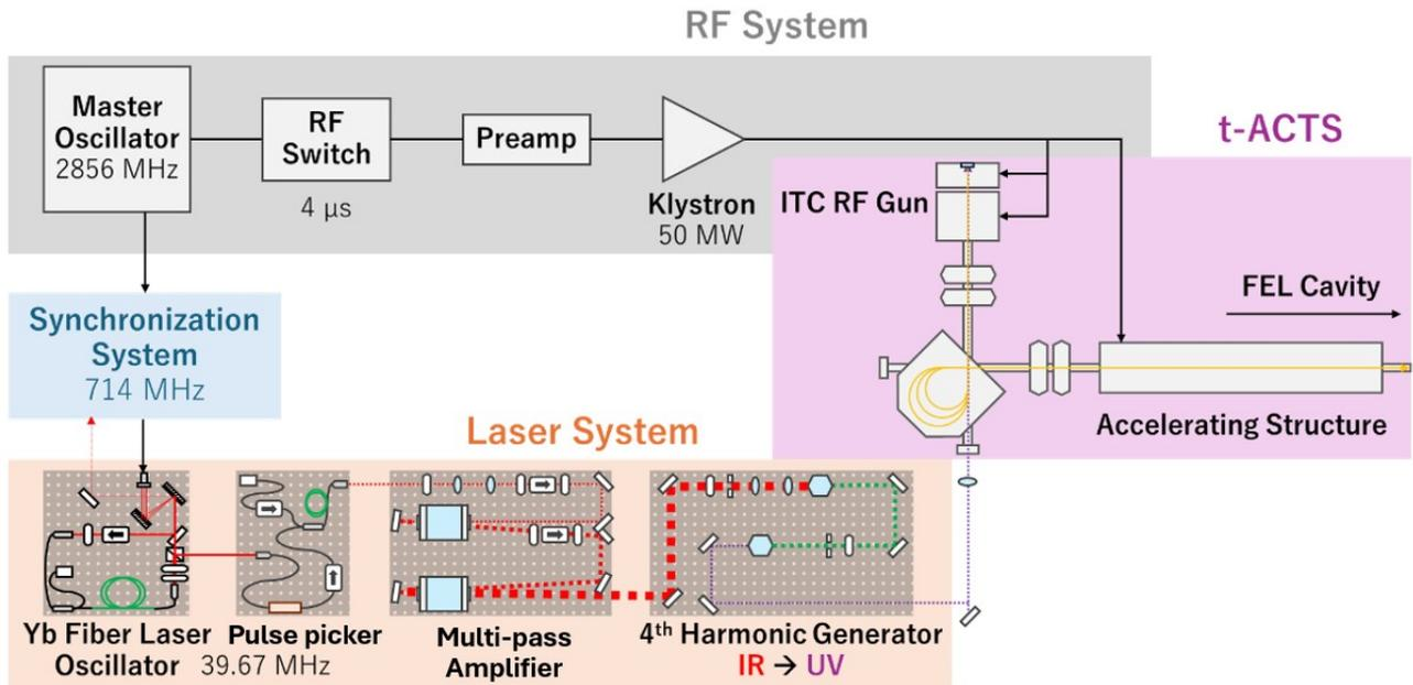
Figure 1: Diagram of the overall systems.
