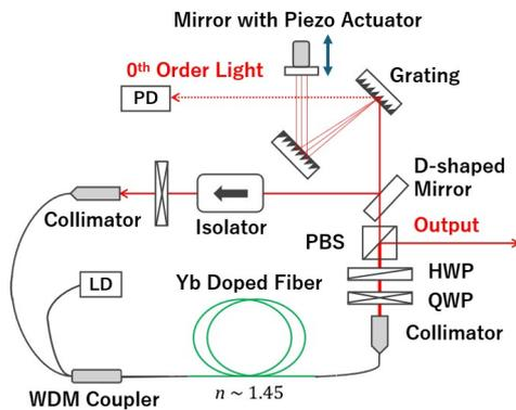
Figure 2: Schematic of a Yb fiber laser oscillator.
