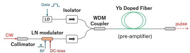
Figure 3: Schematic of a pulse picker section that includes an LN modulator and a pre-amplifier.
