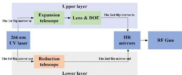
Figure 4: Block diagram of double-layer layout for the 2nd laser line.
