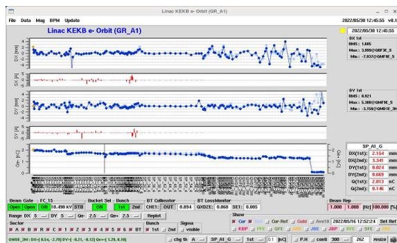
Figure 6: The electron beam orbit for SuperKEKB HER injection in 2022a commissioning.
