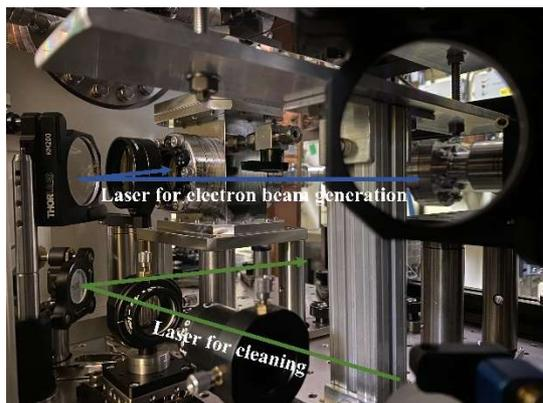
Figure 5: One part of the double-layer experimental setup. Blue line shows the laser for electron beam generation by passing the DOE; the green line shows cleaning mode laser.
