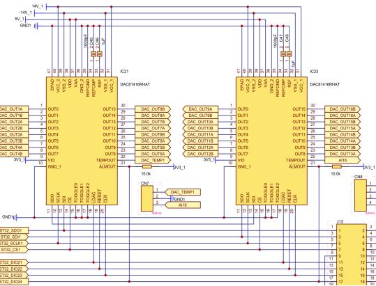
Figure 5: Two DACs are connected in daisy-chain.
