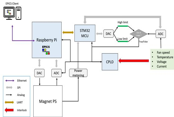
Figure 3: The software schematic diagram.
