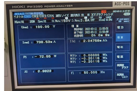
Figure 6: The HIOKI PW3390 power analyzer.
