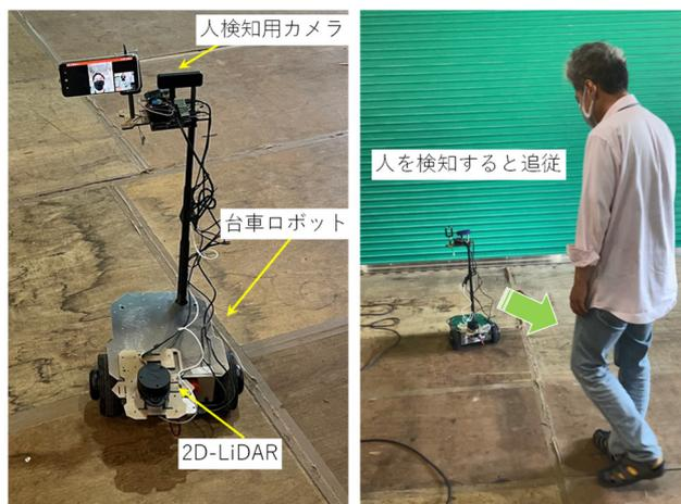
Figure 8: Dolly robot with function to follow person.
