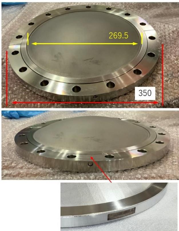
Figure 2: A picture of the beam window with a rotatable flange. Arrangement of both concave (up) and convex (middle) is available. The falling prevention groove is prepared on the side.
