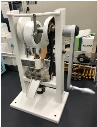
Figure 2: Tabletop tablet press for sample preparation.
