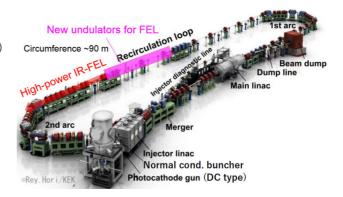
Figure 1: Schematic of the cERL.
