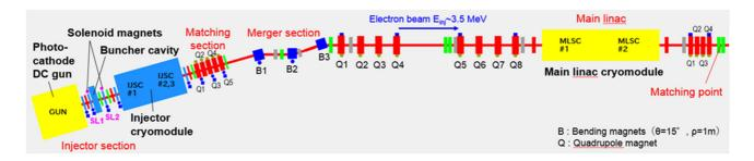
Figure 2: Layout of cERL injector line.
