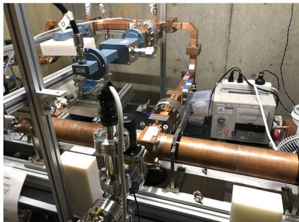
Figure 2: Photo of the main accelerating tube.
