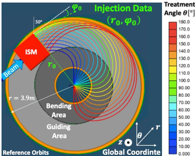
Figure 5: Particle orbits in the midplane of the HTSS Gantry System, using numerical calculation.
