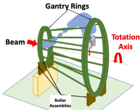
Figure 1: In a traditional gantry system, magnets are mounted in gantry rings and rotated with roller assemblies to acquire planned treatment angles.
