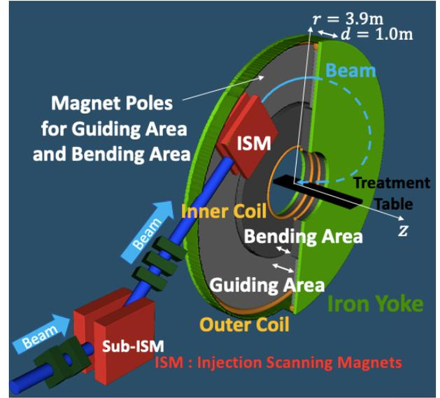
Figure 3: Designed structure of the HTSS Gantry System. Magnets poles for guiding area and bending area are illustrated in light gray and dark gray. Treatment area is within the range of inner coils, where is magnetic field free. Injection Scanning Magnets (ISM) are installed in the HTSS Gantry System.
