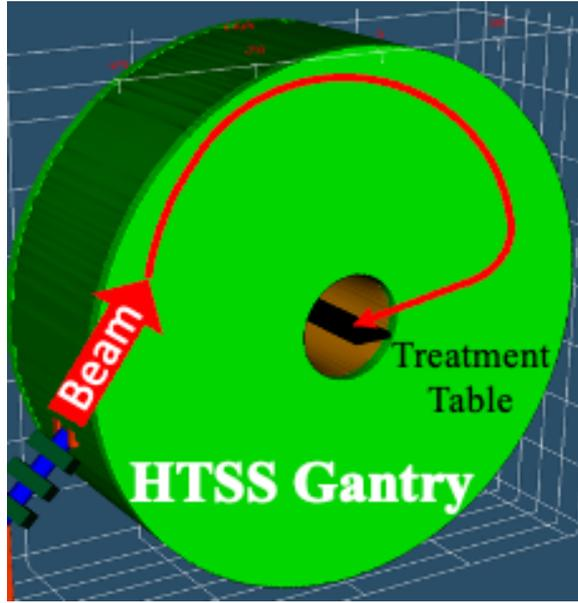
Figure 2: The concept of a HTSS Gantry System. Beam is injected from the left side and transported to treatment table in the center by internal magnetic field. The treatment angle is set by controlling the magnet field.
