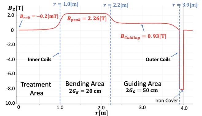
Figure 4: Magnetic field profile in the midplane simulated by OPREA. The peak of  $B_z$  in bending area is about 2.26[T]. In guiding area,  $B_z$  keeps at about 0.93[T]
