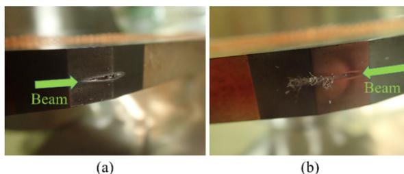
Figure 5: (a) Collimator jaw damaged by beam and (b) that located on the opposite side of (a) where the melted materials are deposited on the surface.
