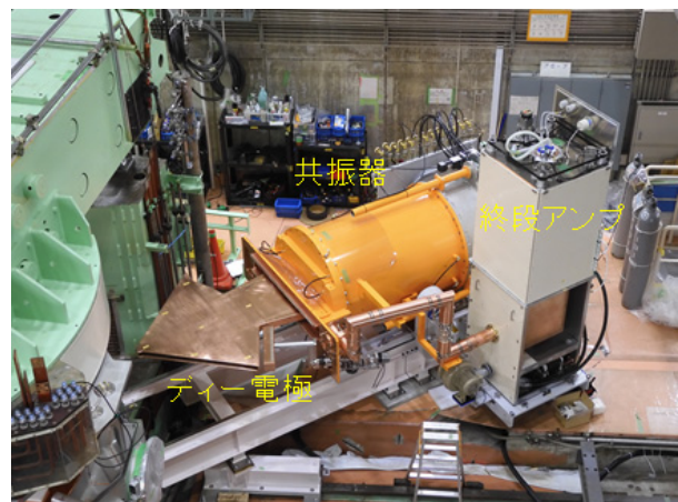
Figure 6: New resonator, Dee electrode and final amplifier after upgrading.
