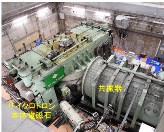
Figure 4: Old AVF cyclotron before dismantling.
