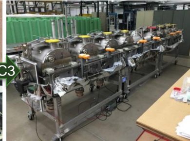
C3 Cold mass ready for baseplate
