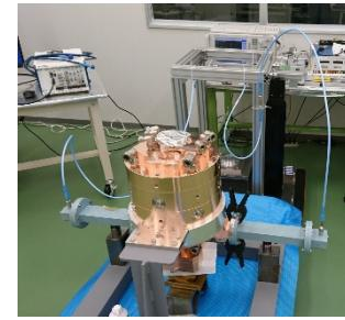
Figure 9: Measurement setup of the SCPC system. The SCPC body is set on a girder and wave guide adapters were mounted by clamping. In the back are seen a network analyzer (straight back) and pulse-response measurement instruments (back left).
