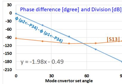
Figure 8: Characteristics of the wave guide mode convertor: measured S-parameters, transmission from MC from the circular wave guide to the rectangular wave guide.
