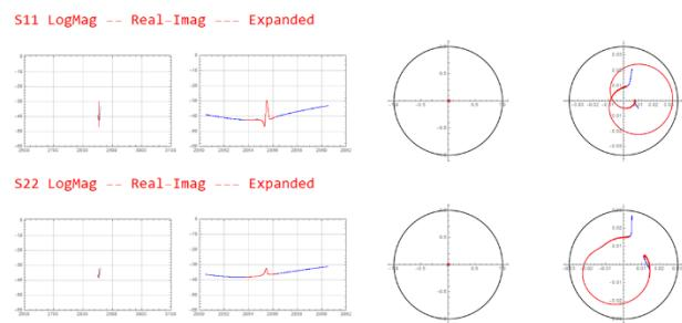
Figure 11: Expanded views of S-parameters of the SCPC system near the resonant frequency of the cavity  $TE_{112}$  mode. The upper row shows  $S_{11}$  and the lower  $S_{22}$ . From left to right, log-mag plots for full spectrum, the same near 2856 MHz, complex-plane plots with unit circle and the magnified complex-plane plots. For all the plots, the red lines show near 2856 MHz, while blue lines for the full-span plots.
