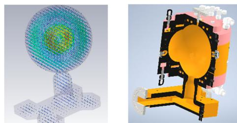
Figure 1: Left: Electric field snap shot of the TE<sub>112</sub> mode of SCPC. Right: Cut view of SCPC.
