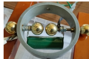
(b) Measurement of pulse current durability
