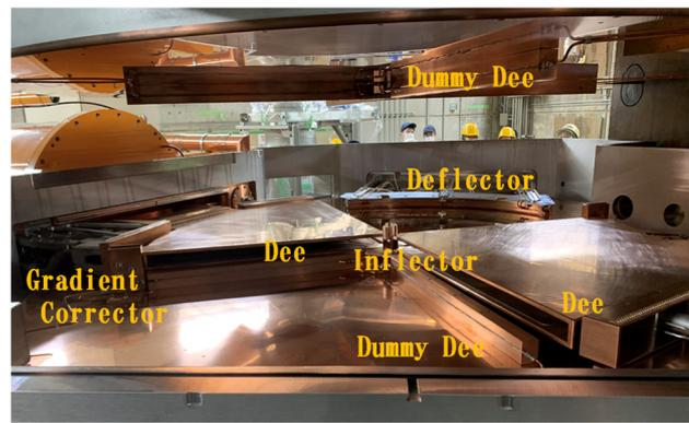
Figure 2: Components inside the AVF cyclotron are shown. After upgrade the upper yoke of magnet can be lifted in 60 cm and then maintainability is achieved.
