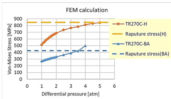
Figure 7: Results of the FEM calculation showing the von-Mises stress as a function of the differential pressure, where 1 atm means 1.013E+5 Pa. Dashed lines show rapture stresses obtained by the tensile test.
