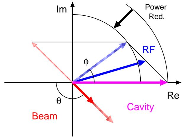
Figure 5: Phase diagram of RF term (blue) and Beam term (red) with phase  $\theta$  after the phase modulation of the input RF with  $\phi$ . The solid and hatched arrows show the instantaneous and the asymptotic values. If  $\theta > \pi/2$ , the input power should be also modulated (less power).
