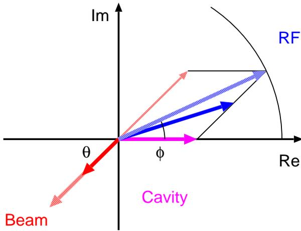
Figure 4: Phase diagram of RF term (blue) and Beam term (red) with phase  $\theta$  after the phase modulation of the input RF with  $\phi$ . The solid and hatched arrows show the instantaneous and the asymptotic values.
