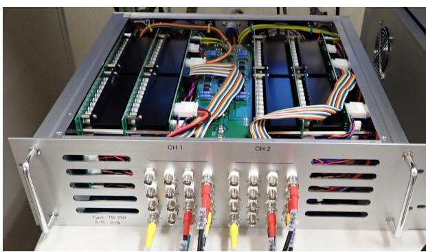
Figure 3: Type TB-250 Bipolar power supply for pulsed steering magnet.
