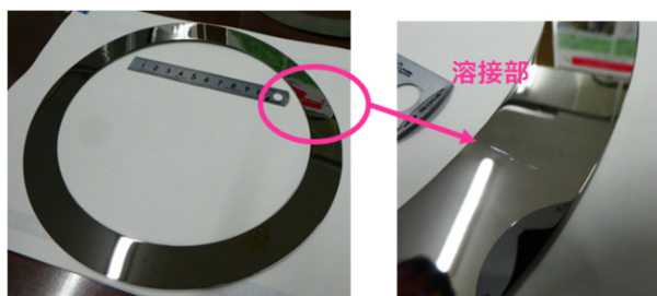
Figure 5: Photographs of the diaphragm made from a 45-degree welded plate.
