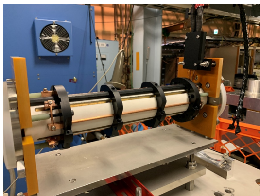
Figure 10: photo of CCI PM on test bench.
