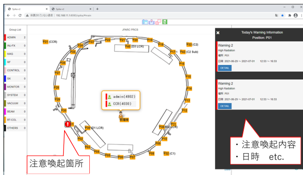
Figure 10: Function to push notifications such as high radiation areas and magnet operation tests.
