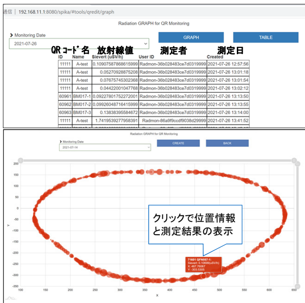
Figure 7: Listing and plotting of radiation measurement results.
