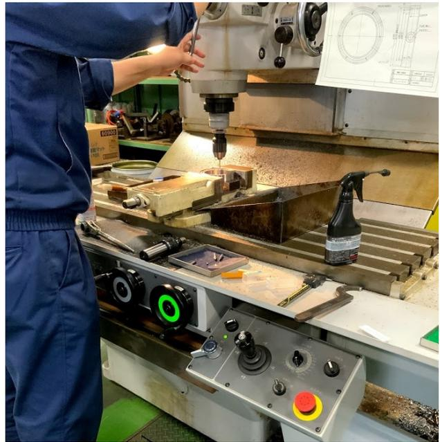
Figure 3: Processing of a vacuum chamber using a CNC milling machine at the Ibaraki KOSEN workshop.
