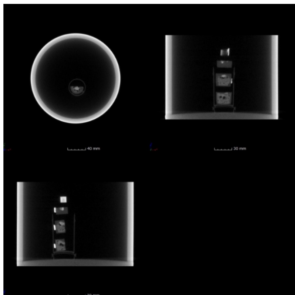
Figure 6: Reconstruction result of simulated debris in thick-wall storage can using 3.95 MeV CT.
