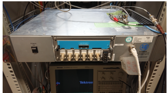
Figure 1: LLRF box. The BNC connectors in the front panel are auxiliary inputs to the RTM.
