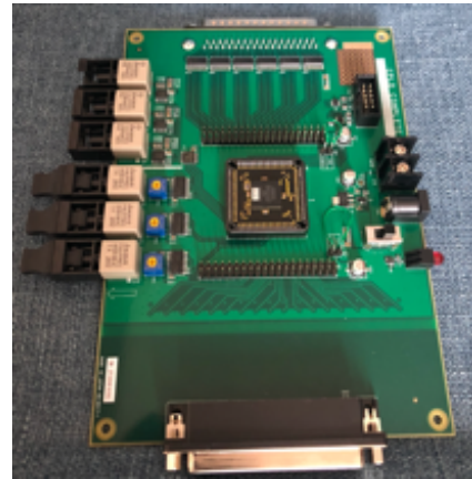
Figure 11: Adder board we have designed for the beam experiment using one half-arc of MR.
