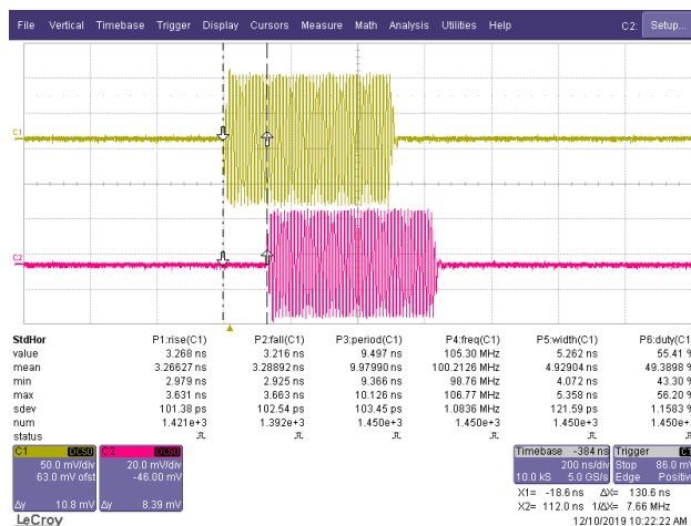
Figure 10: Delay time measurement between input and output @4.096GSPS.
