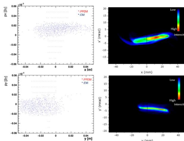
Figure 5: Calculated (left) and measured (right) beam phase space distribution at EM in the condition of  $\pm 2$  mm of the slit width after HECR for 17.04 keV  $^4\text{He}^{2+}$ . The calculated distributions for PPEM (red dot) and EM (blue dot) were obtained by OPAL-T code.
