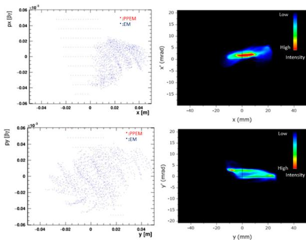
Figure 4: Calculated (left) and measured (right) beam phase space distribution at EM in the condition of  $\pm 10$  mm of the slit width after HECR for 17.04 keV  $^4\text{He}^{2+}$ . The calculated distributions for PPEM (red dot) and EM (blue dot) were obtained by OPAL-T code.
