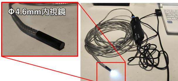
Figure 5: The photograph of the endoscope of which the diameter is 4.6 mm and its cable length is 5 m.
