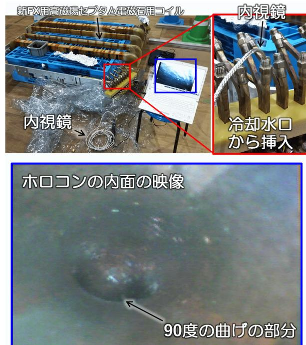
Figure 6: The observation of the inner side of the magnet coil of the FX Septum magnet by the endoscope.
