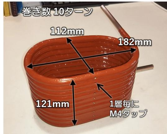
Figure 2: The photograph of the test-coil for study the impedance of the layer-shortened coil.
