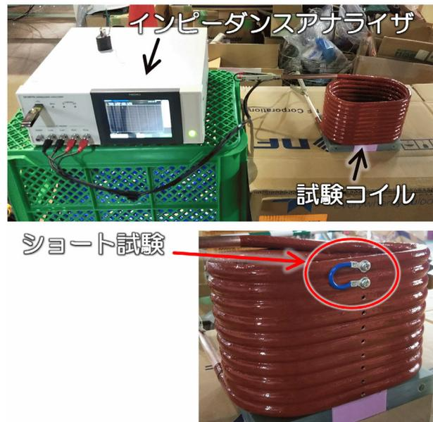
Figure 3: The photograph of the setup of the measurement of the impedance and inductance of the test-coil.
