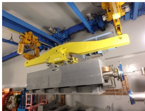
Figure 10: Photograph during an installation of the Lambertson magnet with the long-stroke pillow-seals.
