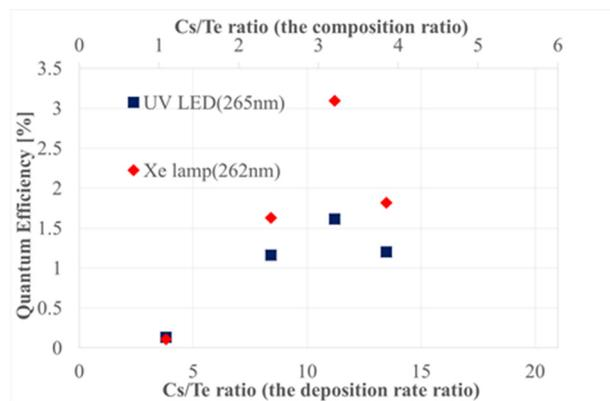
Figure 4: The relationship between Cs/Te ratio and Q.E.
