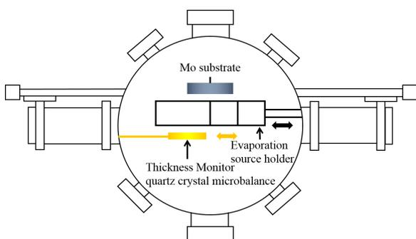
Figure 2: Schematic of the photocathode evaporation system.
