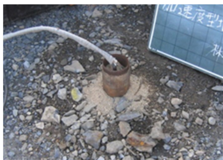
Figure 2: Accelerometer placed on ground surface.
