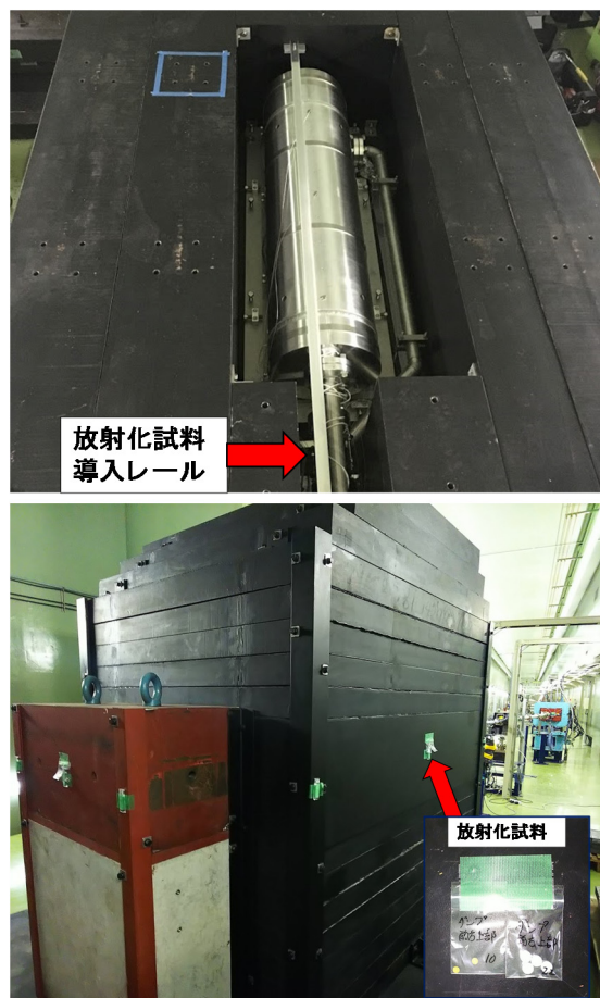
Figure 7: Setting of gold foil and aluminum pellet. (a) Inside shield. (b) Outside shield.
