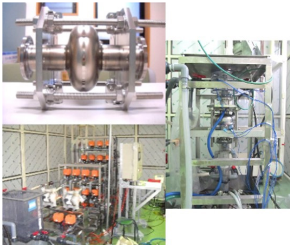
Figure 1: Photos of single cell cavity TB1-TSB02 (upper left), VEP facility (lower left), cavity setup (right).
