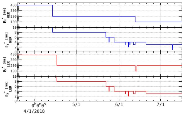
Figure 3: History of beta squeezing in the Phase 2 commissioning. The blue lines for the HER and the red lines for the LER.
