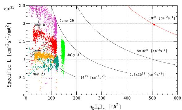
Figure 5: Specific luminosity as a function of bunch current product multiplied by number of bunches. Plots except for green dots indicate the reference beam currents and bunch numbers. The green dots indicate the high bunch current operation.
