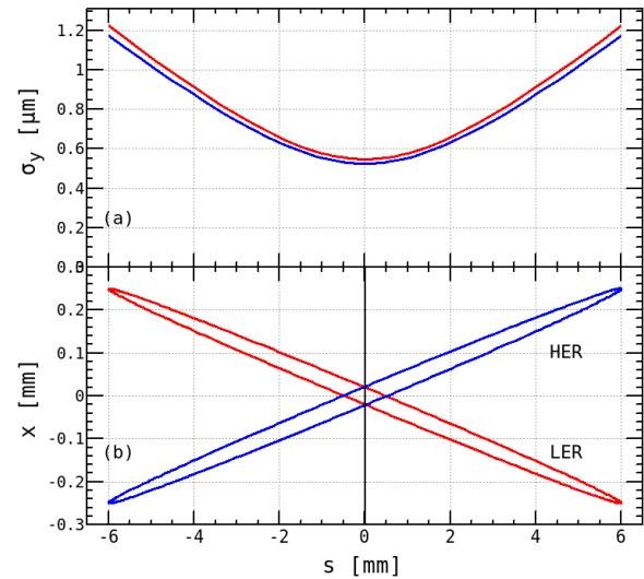
Figure 1: (a) Beam spot-size in the vertical direction in the vicinity of the IP. (b) Top view of the colliding bunches with a large crossing angle. The ratio of vertical emittance to the horizontal emittance is assumed to be 5% in the LER and 2% in the HER.
