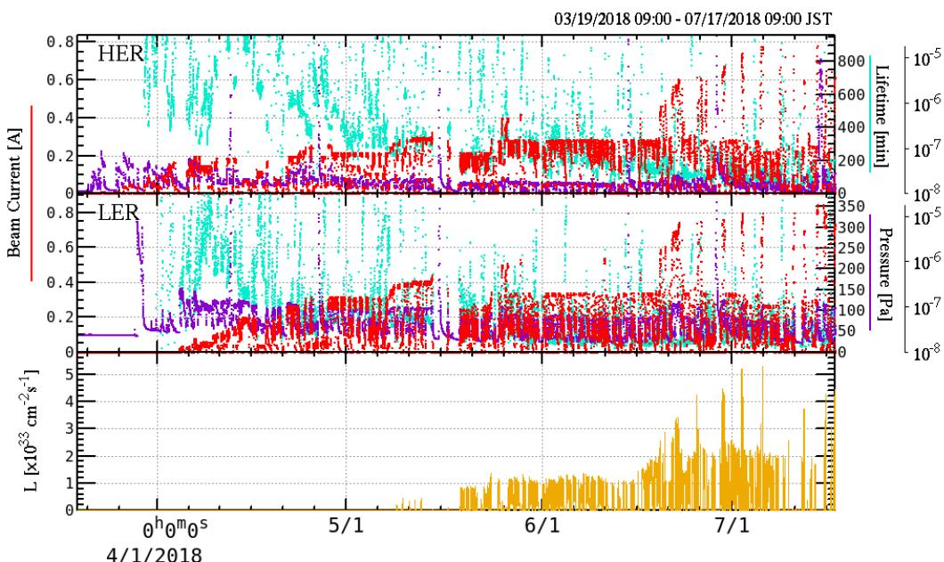
Figure 2: History of Phase 2 commissioning. The red points indicate the beam current, cyan for the beam lifetime, purple for the average vacuum pressure. The luminoosity is indicated by yellow.
