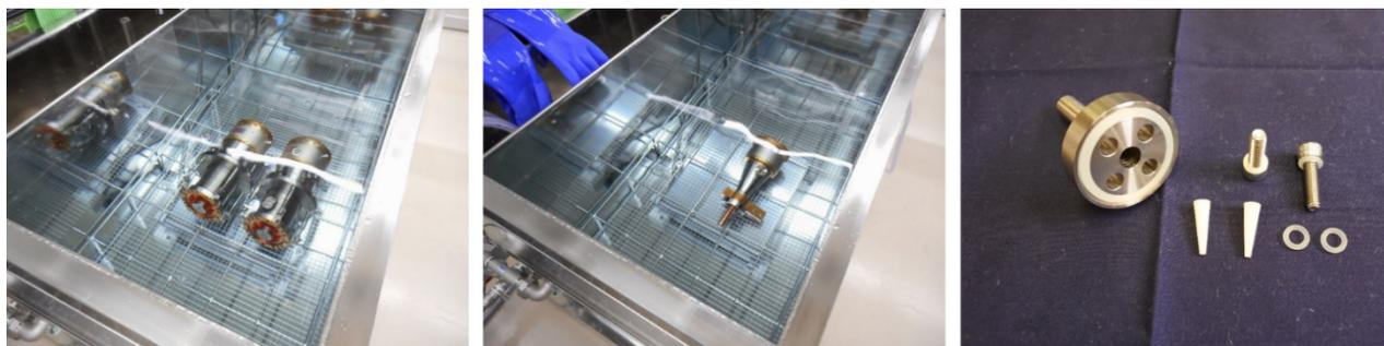
Figure 1: Power couplers in the ultrasonic rinsing bath at TETD (Left: Warm parts, Center: Cold part, Right: Waterproof parts). The maximum power of ultrasonic rinsing for warm parts was 360 W to avoid the removal of TiN coating from TiN coated ceramics used for warm windows.
