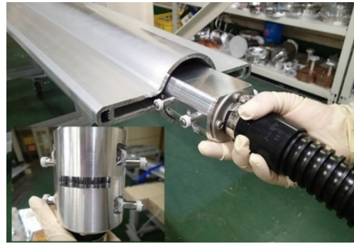
Figure 13: Special tool for collecting dust particles at the bottom of beam channel.
