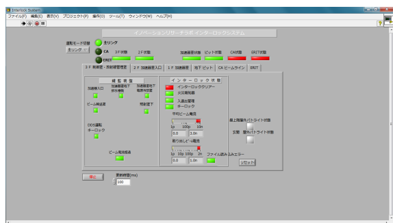
Figure 3: Operator interface for the interlock control based on LabVIEW.
