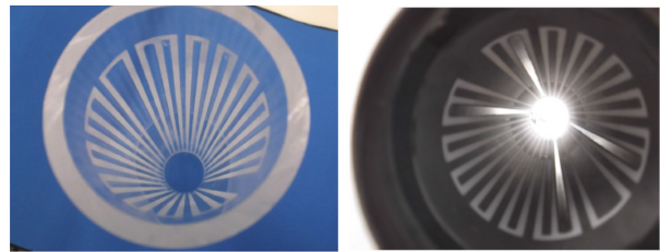
Figure 7: A precise pattern coating on the PVC pipe and the ceramics chamber by masked-blast technique.
