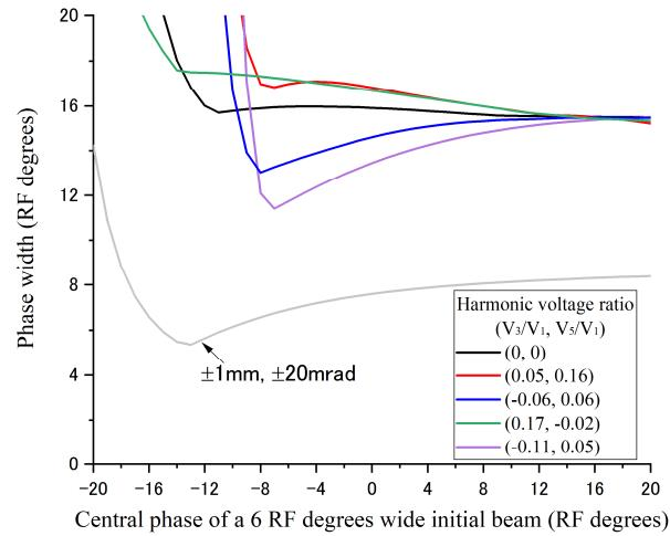
Figure 4: Calculated phase width using the harmonic acceleration with the geometrical orbit analysis model for the  $\text{H}^+$  20MeV condition.
