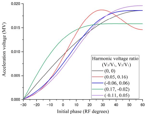
Figure 3: Calculated acceleration voltage waveform at the first acceleration gap for the  $\text{H}^+$  20MeV condition.
