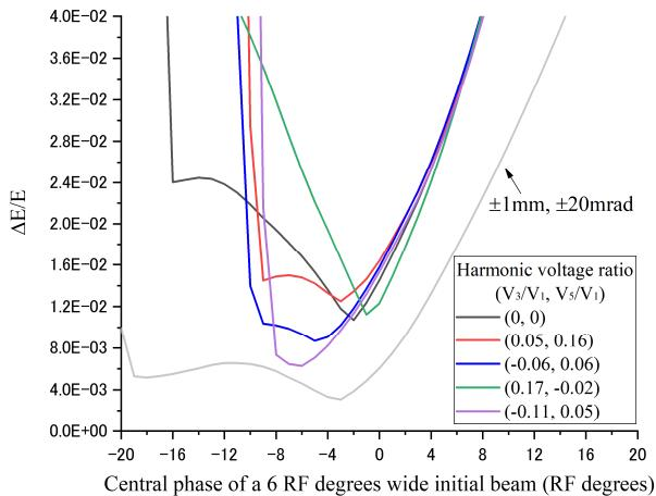
Figure 5: Calculated energy spread using the harmonic acceleration with the geometrical orbit analysis model for the  $H^+$  20MeV condition.
