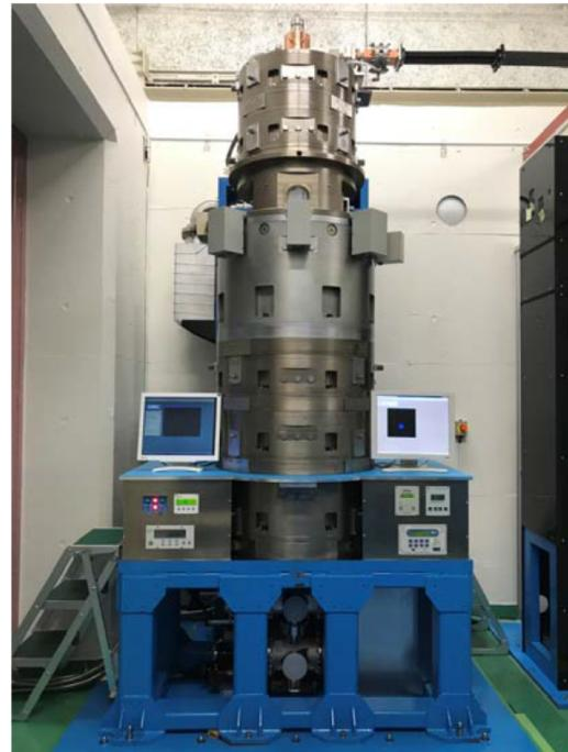
Figure 5: Ultrafast electron microscopy using relativistic-energy femtosecond electron pulses.
