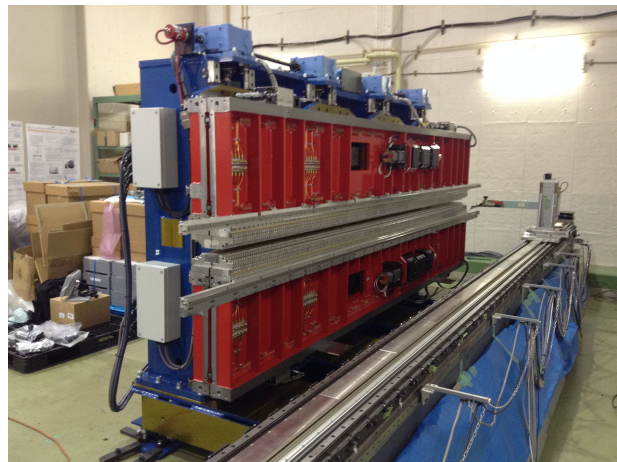
Figure 2: New insertion device for BL19.
