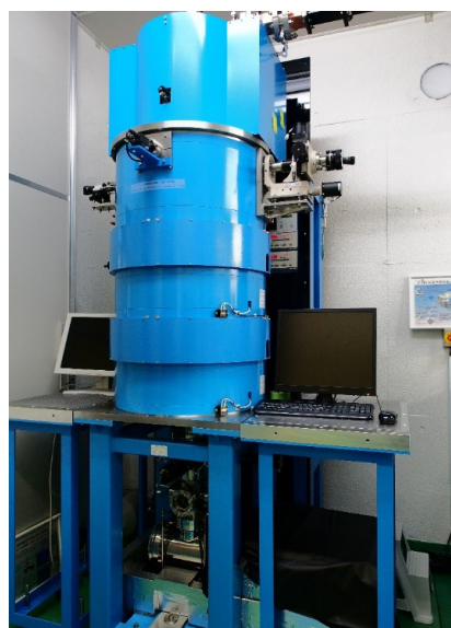
Figure 1: The prototype relativistic ultrafast electron microscopy using a photocathode rf gun.
