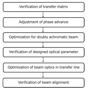
Figure 2: Flow chart of verification and optimization of beam optics.
