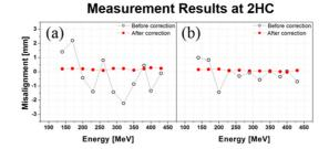
Figure 6: Measurement results of the beam misalignment. Horizontal (a) and vertical (b) misalignments at 2HC before correction (open circles) and after correction (filled circles).
