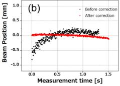
Figure 3: Verification of the transport matrix(a) and dispersion function(b).
