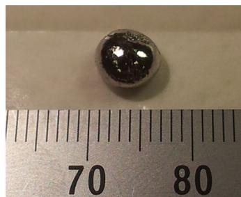
Figure 3: Photo of Ir<sub>2</sub>Ce ingot.
